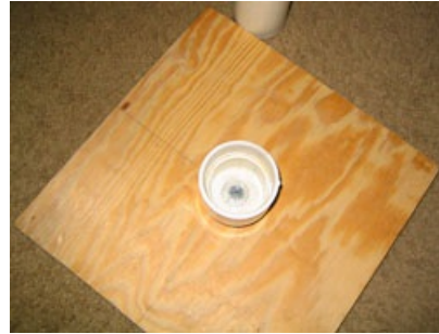
Note the counter sink allows the carriage bolt to be flush (or recessed) with the bottom of the foot.
